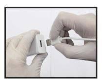
Connect the charging cable (Micro 5pin USB) to the universal USB charger.
