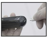
Connect the charging cable (Micro 5pin USB) to the charging port.
